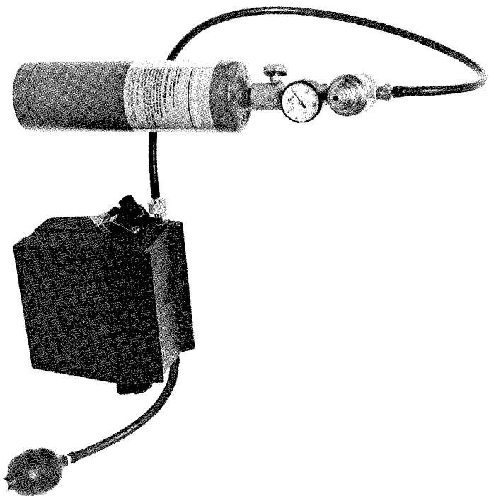
Figure 5-2. Connection of Calibration Equipment
