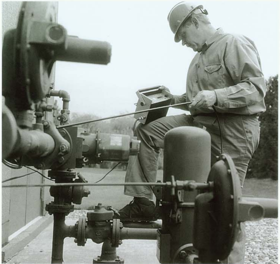
By attaching probes and lines to the Watchman Multigas Monitor, workers can test remote areas or confined spaces before entry.
